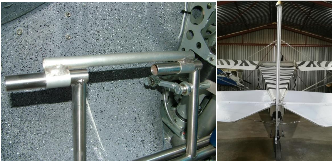
Figure 2.3.4.1: (a) Control surface alignment jig, (b) Rudder neutral position
