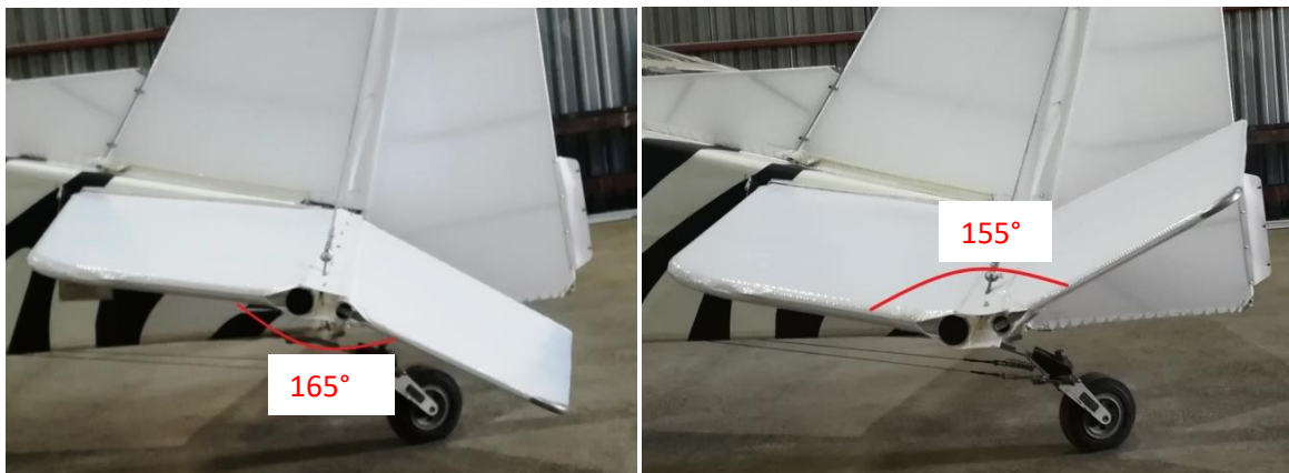
Figure 2.3.3.2: (a) Full nose down deflection position, (b) Full nose up deflection
