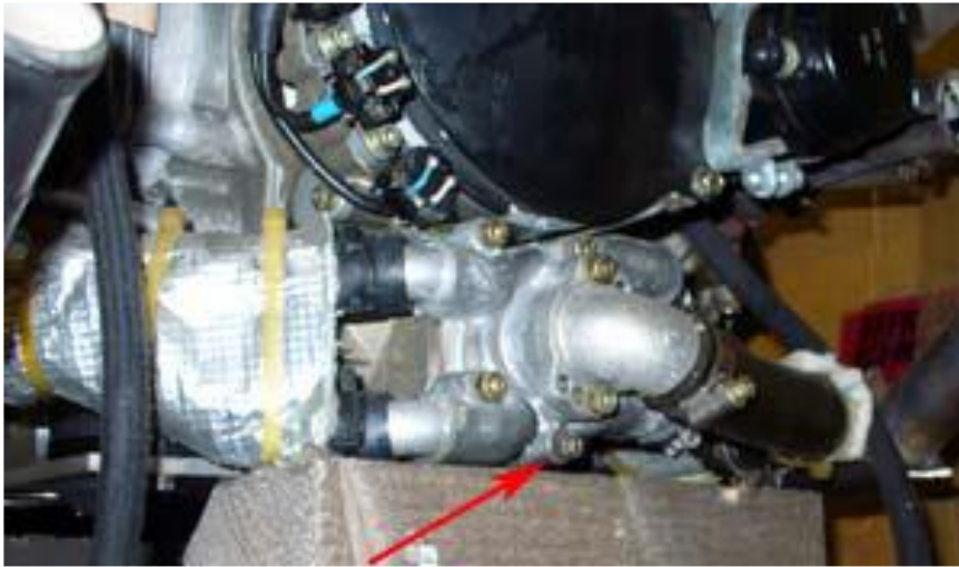
Figure 2.8.1.1: Water drain screw on the water pump
