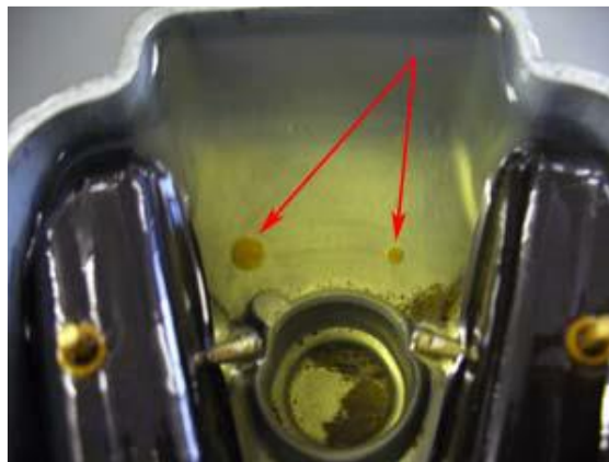
Figure 2.6.4.2: Water evident in the float bowl
