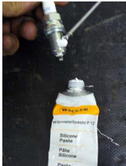
Figure 2.5.7.1: Applying heat conduction compound
