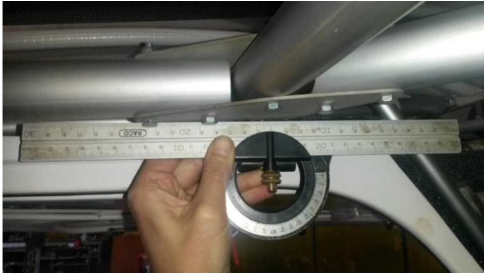
Figure 2.1.1.2 – Aircraft longitudinal angle determination
