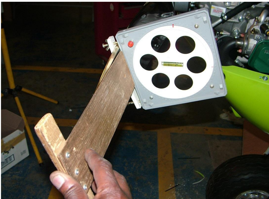
Figure 2.9.1.3: Fitting the inclinometer to the blades
