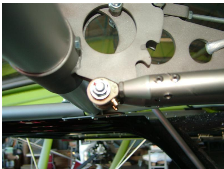
Figure 2.3.2.1: Flap push rod adjustment
