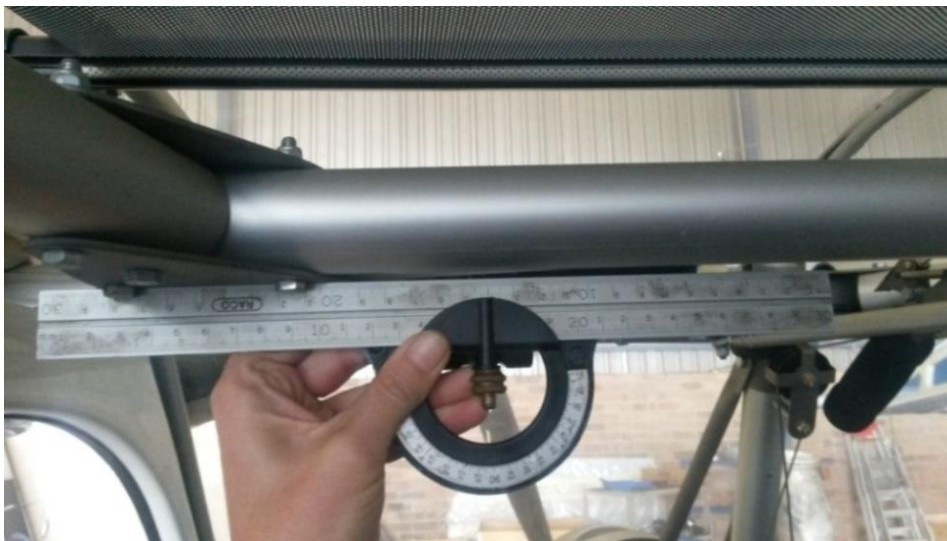
Figure 2.1.1.1 – Aircraft lateral angle determination
