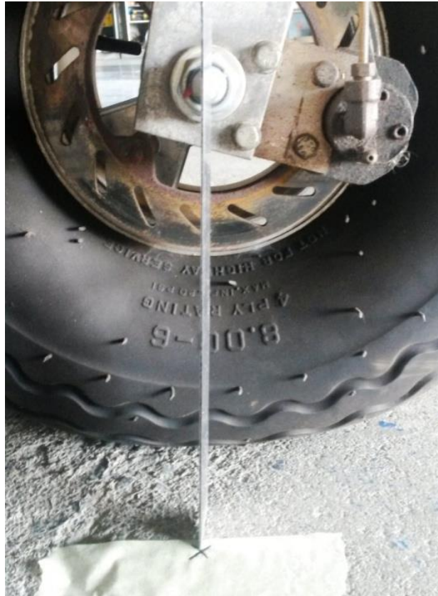
Figure 2.1.1.4 – Point directly below the centre of the axle
