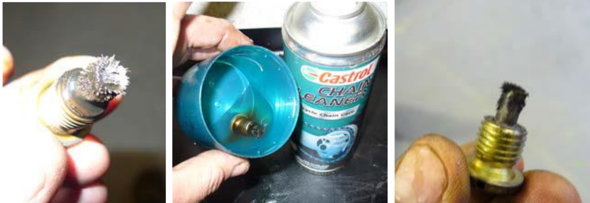
Figure 2.5.5.2: (a) Magnetic plug contaminated with oil and iron filings, (b) Cleaning the plug & (c) Plug after cleaning still showing iron filings
