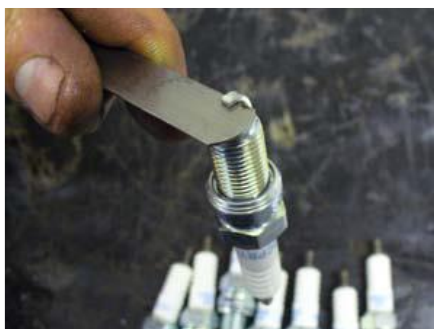
Figure 2.5.6.1: Checking of the gap using a feeler gauge
