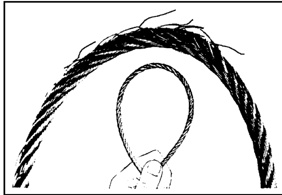
Figure 2.1.9.1 – Cable inspection technique
