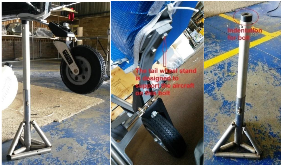
Figure 2.1.2.4 – (a) Tail wheel stand, (b) position on aircraft and (c) stand
