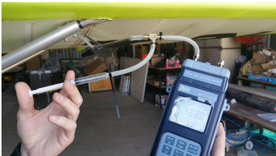
Figure 2.10.1.1: Arrangement of instrument calibration system
