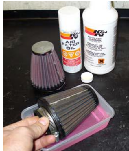
Figure 2.5.2.2: Applying oil to the engine air filter
