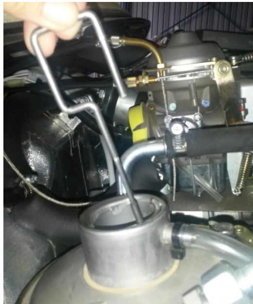
Figure 2.7.1.2: Removing the dipstick
