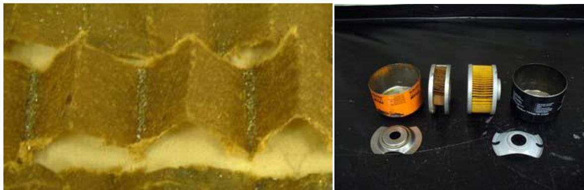
Figure 2.7.2.4: (a) Contaminated filter paper and (b) Copy filter (left) and genuine Rotax filter (right)
