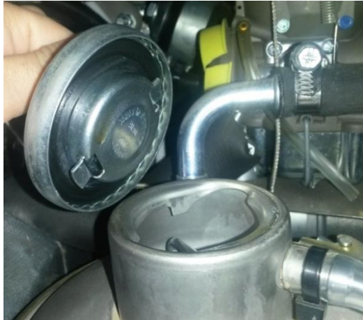
Figure 2.7.1.1: Removing the cap from the oil tank
