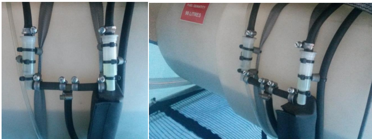
Figure 2.6.2.1: Fuel filter position on aircraft fuel tank
