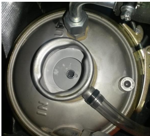
Figure 2.7.1.3: Opening for pouring the oil in
