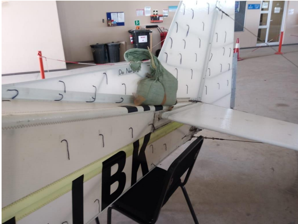
Figure 2.1.2.3 – Raising the nose gear by positioning weights on the tail on a cushioned chair
