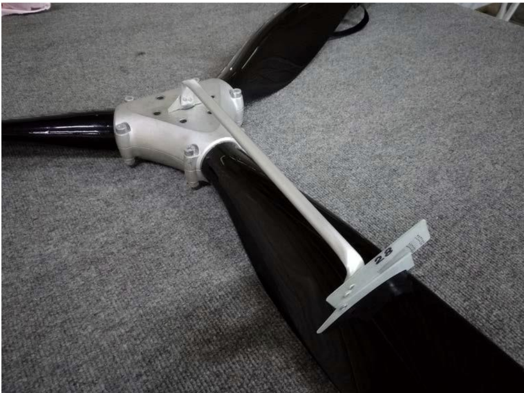
Figure 2.9.1.2: Kiev pitch setting tool
