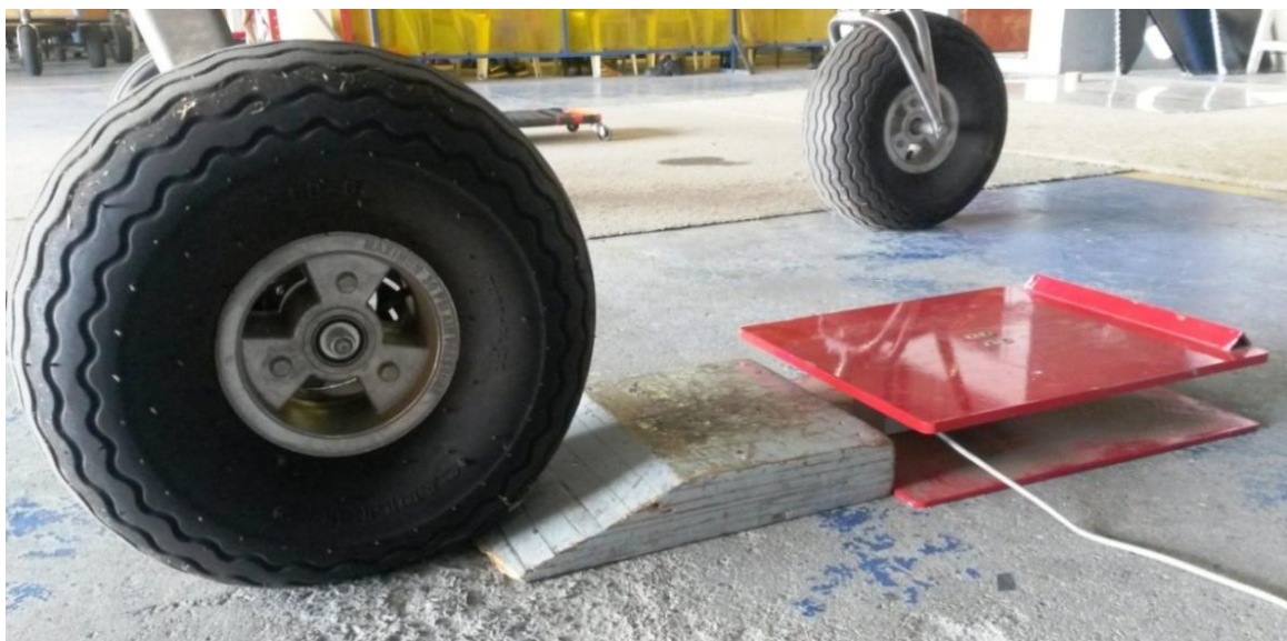
Figure 2.1.1.5 – Aligning the scales with the aircraft wheel
